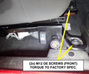
Re-attach the OE screw securing the seat belt to the side of the seat using a T45 Torx bit. **Torque to Factory Specification**
