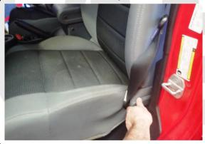
Unplug any cables attached to the seat. The number and type of plugs will be model and year dependent. (JK JEEP 2007 RH Drivers Side Shown)
