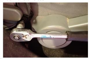
Carefully remove the head rest from the seat, and the seat from the vehicle and place on a clean work surface, taking care to keep the sliding seat tracks in their original aligned positions. *HINT:* Release the door strap from its post to enable a wider door opening if required, prior to seat removal (Don't forget to reconnect it later).
